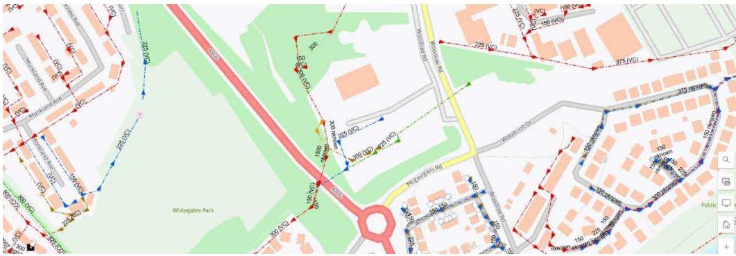
Figure 2 –extract from Scottish Water Asset Plans indicating surface water sewer serving the new Aldi site discharging into an open ditch and pond which in turn connects into the South Catchment Outfall. Does the maintenance of this open ditch rest with Scottish Water or the Council? It is important that the full length of this upstream catchment pipe is surveyed to confirm all existing connections contributing to the overall flow; this has not been done. For example, the building shown to the north of the new Aldi site will have substantial and un-attenuated surface water run-off discharging either into the adjacent combined sewer or it may be linked to the culvert upstream of the surface water sewer, and thus it may not have been modelled in the design calculations or the FRA.
